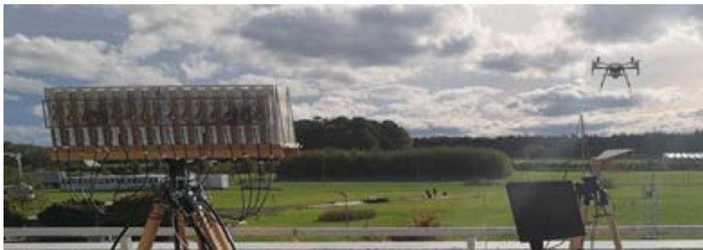
(c) Passive Radar for the Detection of Small Objects
