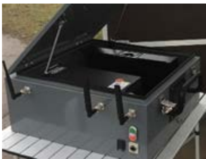
(a) Detector for Drone-Type Radio Signals
